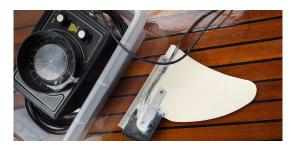
The same transducer mounted together with a plastic fin on a nylon block which slides in the rails at the bottom of a SUP board. Approx 5 cm has to be added to get SDDBS
