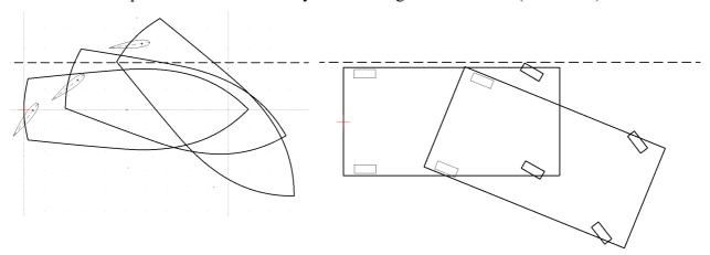
Please note that there must be **enough room at the stern** to turn a ship. This is clearly different from a car, where a steering action moves the **front** sideways
