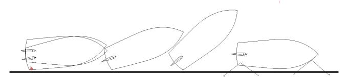
A person on the shore loosens the ship, except for the stern line, and presses it an arm's length away. Then he/she pulls the stern back close to the quay and pulls the stern **forward along the quay** with the stern line (with the stern as close as possible to the quay). While doing so the bow will turn further and further out. Get on board at the last minute and sail away **with the rudder straight**.
