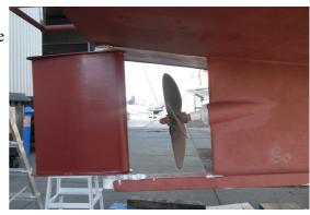
reduced. For sailing yachts with a short keel and large seagoing ships, this is usually not done and one sees thicker rudder shafts.
