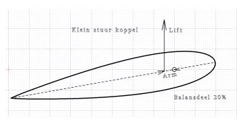
Without specific computer simulations or tests, I would not choose a larger balance part than 20% for small vessels. The mentioned (lift) distance of (0.25 x length), is after all a measured value and concerns a test set-up with an even flow. This is not necessarily equivalent to the actual situation. The propeller for example, rotates at a short distance in front of the rudder.
