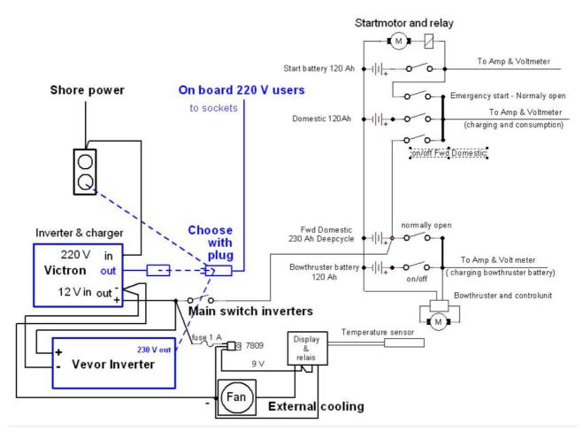
In the morning, before the sun can start charging and after an evening with the use of TV and possibly the stove, the battery voltage is usually at its lowest. Especially after a few days with little sun, the voltage can have dropped quite a bit. If one sails away at such times, it is wise to avoid the use of the bow thrust-er, windlass or other large users, if possible.
