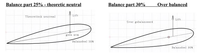
In the case of large shipbuilding, larger than 20% balance percentages are used, but larger forces play a role that one wants to avoid and heavy hydraulic steering machines are used to control a rudder. Also specific tank test and/or computer simulations are carried out beforehand.
