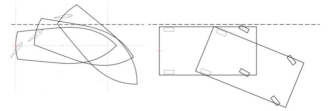
Please note that there must be **enough room at the stern** to turn a ship. This is clearly different from a car, where a steering action moves the **fron**t sideways
