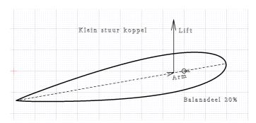
Without specific computer simulations or tests, I would not choose a larger balance part than 20% for small vessels. The mentioned (lift) distance of (0.25 x length), is after all a measured value and concerns a test set-up with an even flow. This is not necessarily equivalent to the actual situation. The propeller for example, rotates at a short distance in front of the rudder.
