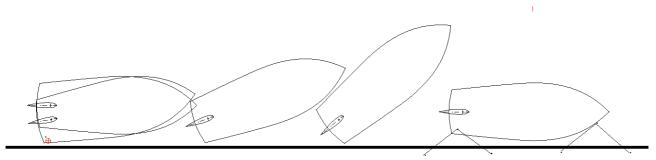
A person on the shore loosens the ship, except for the stern line, and presses it an arm's length away. Then he/she pulls the stern back close to the quay and pulls the stern **forward along the quay** with the stern line (with the stern as close as possible to the quay). While doing so the bow will turn further and further out. Get on board at the last minute and sail away **with the rudder straight**.
