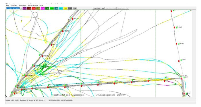
The lateral buoys indicates the lateral boundary of the waterway. The depth in these waterways should be at least 1.7 m (yellow or grey measuring points)
