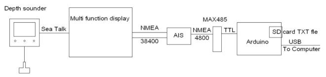
When the MFD and AIS function correctly, the depth information from the sounder is delivered to the MFD via the SeaTalk connection and from the MFD via NMEA 38400 baud to the AIS.
